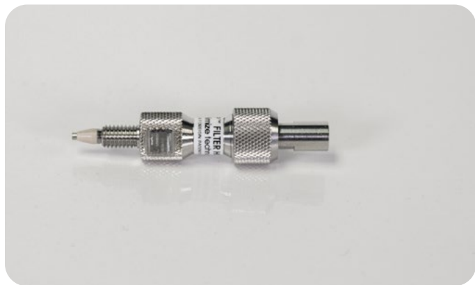
Figure 4. Direct connect guard cartridge. This type of guard column does not require any connecting tubing to connect to the analytical column; it screws right into the column inlet (see also Figure 6 ).
