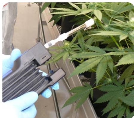
**Figure 3.** Indoor profile measurement of cannabis terpenes (flowering plant) from cannabis greenhouse growing operations using a glass Carbotrap® T420 TD tube and detector tube pump.
