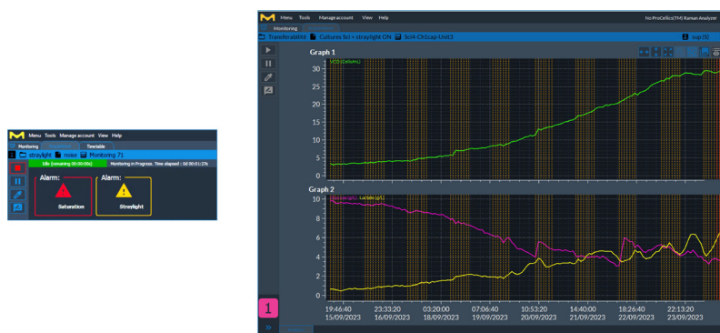
Figure 3: Bio4C® PAT Raman Software reporting alarms for straylight and saturation detection during batch monitoring
