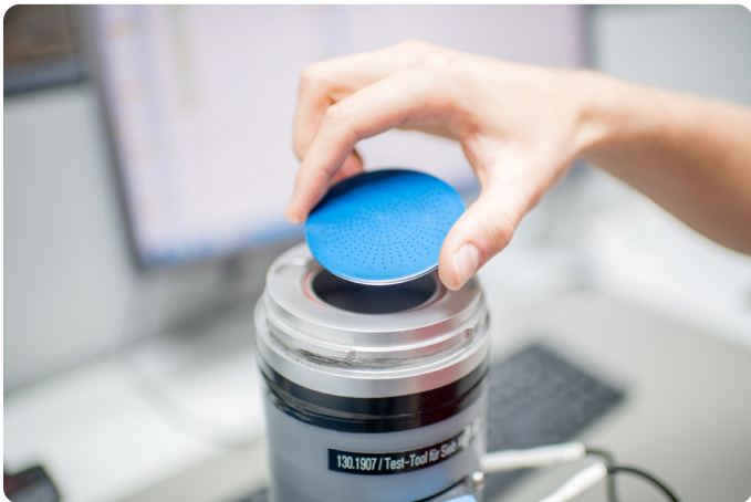
Figure 7: An aluminum sieve is tested for airflow as the anodization has an influence on the hole diameter and therefore on impaction speed.
