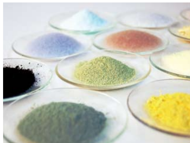
Figure 1. Using flame spray synthesis, the compositional variety of inorganic nanoparticles is nearly endless. Different oxitic, salt and metallic nanoparticles with similar particle size distribution are depicted (courtesy of Nanograde LLC.).
