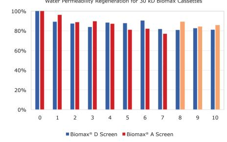
Water Permeability Recovery after Cleaning; Cassettes with 30 kD Ultracel® Membranes with C, D and V Screen
