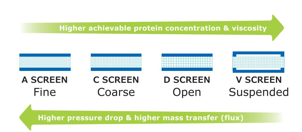
To address this tradeoff, a new cassette was developed that uses an open "D" screen as well as special internal channel design optimization to reduce pressure drop while also maintaining a high mass transfer coefficient. As a result, it can achieve the high protein concentration of more open channels while maintaining the high flux and low membrane area of tighter channels.
