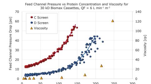
Feed Channel Pressure Drop versus Protein Concentration and Viscosity for Cassettes with 30 kD Ultracel® Membranes with C, D and V So
