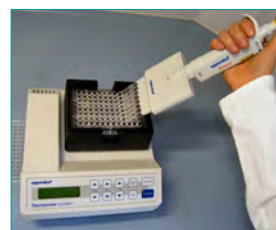
6. Washing (removal of unbound components, 2x1min)
