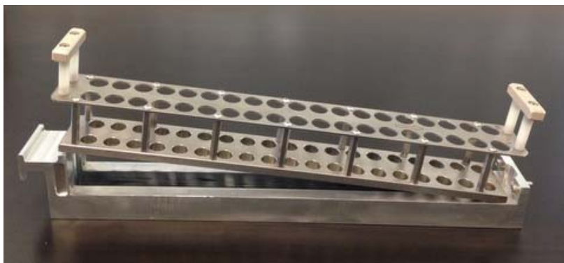
Figure 2 – Adding Metal Rack to Base
