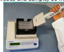
7. Washing (Removal of unbound components, 2x1 min)
