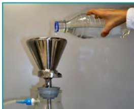
1. Sample filtration (100- 1000 ml water, 15 min)
