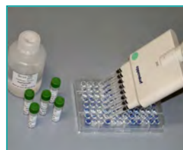
8. Encymatic reaction (Enzymatic colour reaction, 5-15 min)
