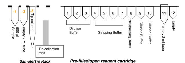
The Buffer Arrangement in Pre-filled Cartridges and Tubes:
