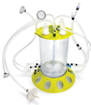
Figure 1. Opticap® XL 50 Capsules with Millipore Express® SPG Hydrophobic Membrane installed on a Mobius® CellReady 3L Bioreactor.
