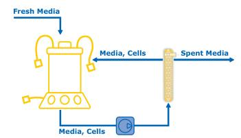
Figure 1: Cellicon<sup>™</sup> filter connected to 3 L Mobius<sup>®</sup> bioreactor.
