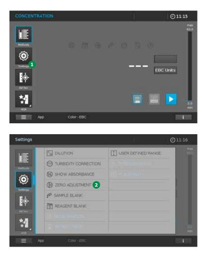
If a valid zero adjustment is already available, the Methods window opens. The zero-adjustment procedure must then be selected by opening **<Settings>** 1 and clicking on the selection button **"ZERO ADJUSTMENT"** 2.
