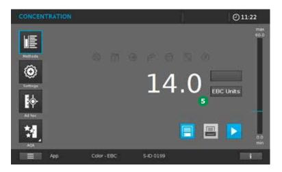
• Fill the sample solution into a 10-mm rectangular cell and insert the cell into the cell compartment. The measurement is performed automatically and the result appears in the display **5**.
