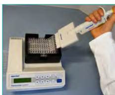
4. Immobilisation (Binding of the „sandwiches“ to the binding plate, 10 min)
