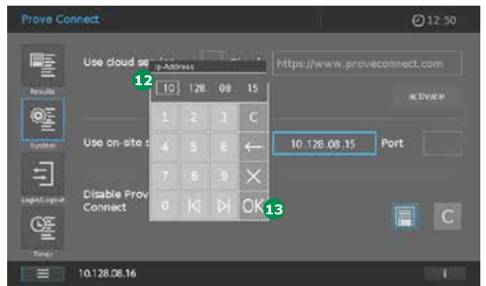
Figure 40 - Screen of Spectroquant® Prove / Prove plus (Figure 37) with entered IP address of the PC on which Prove Connect runs
