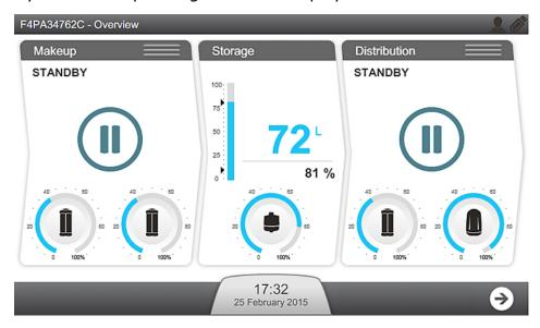
**Important:** Standby should only be used to stop the corresponding process in the event of a leak.
