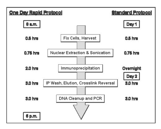
Comparison of the Rapid Magna ChIP<sup>TM</sup> and Standard protocols. The protocols vary only in the time required for immunoprecipitation. The example of the Rapid Protocol shown above is only recommended for experiments with a limited number of samples. For additional guidelines on selecting the appropriate protocol, see detailed instructions on page 9.
