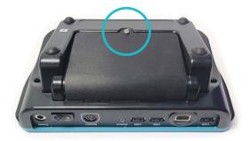
2. The battery pack is mounted to the base of the instrument. Remove the battery pack from the instrument by pulling up on the battery pack tab. This will decouple it from the instrument and lift the battery pack up.
