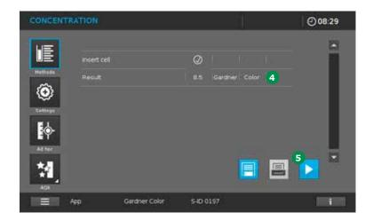
The measurement result appears in the photometer display  $\mathbf{4}$ .
