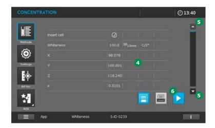
The measurement results appear in the photometer display 4.
