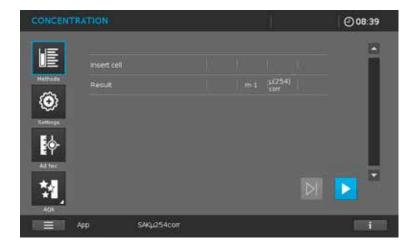
• Fill the sample solution into a corresponding rectangular quartz cell and insert the cell into the cell compartment. The measurement is performed automatically.
