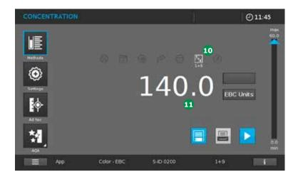
The window changes to the methods display. The activated dilution factor appears in the display  $\mathbf{0}$  and is automatically taken into account in the calculation of the result  $\mathbf{0}$ .
