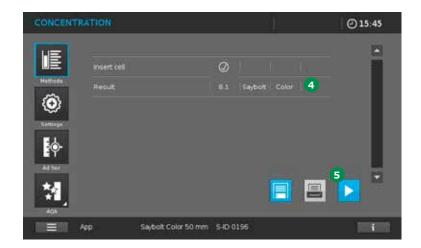
The measurement result appears in the photometer display 4.
