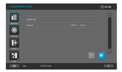
• Fill the sample solution into a 10-mm rectangular cell and insert the cell into the cell compartment. The measurement is performed automatically.
