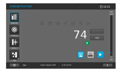
• Fill the sample solution into a corresponding rectangular cell and insert the cell into the cell compartment. The measurement is performed automatically and the result appears in the display 5.
