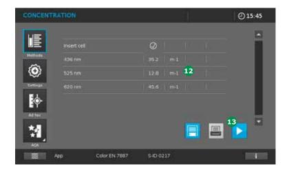
The measurement results at the wavelengths 436 nm, 525 nm, and 620 nm appear in the photometer display ①.
