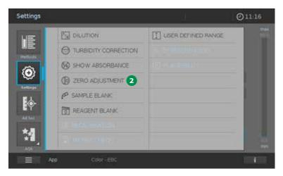
If a valid zero adjustment is already available, the Methods window opens. The zero-adjustment procedure must then be selected by opening **<Settings>** 1 and clicking on the selection button **"ZERO ADJUSTMENT"** 2.
