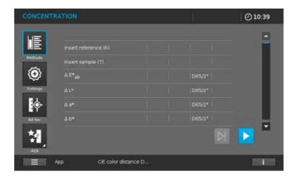
• Fill the reference solution into a 10-mm rectangular cell and insert the cell into the cell compartment. The measurement is performed automatically.
