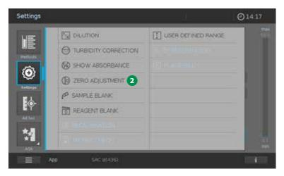
If a valid zero adjustment is already available, the Methods window opens. The zero-adjustment procedure must then be selected by opening **Settings** and clicking on the selection button **ZERO ADJUSTMENT**.
