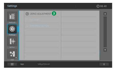
If a valid zero adjustment is already available, the Methods window opens. The zero-adjustment procedure must then be selected by opening **Settings** and clicking on the selection button **ZERO ADJUSTMENT**.
