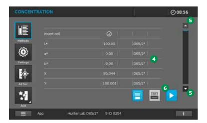
The measurement results appear in the photometer display  $\mathbf{4}$ .
