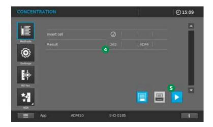
The measurement result appears in the photometer display 4.
