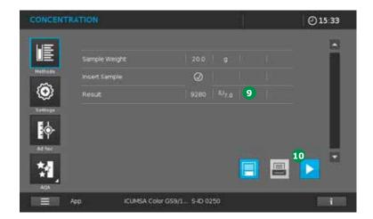
The measurement result in the units  $IU_{7.0}$  appears in the photometer display 9.
