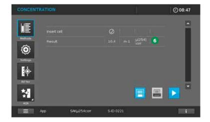
The measurement result appears in the photometer display 6.
