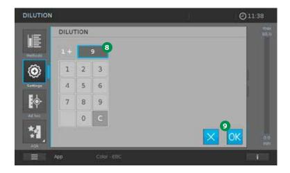
A window with an input field to enter the dilution factor is opened. Activate the input field behind the "+" character  $^{\$}$  and enter the dilution factor in the ratio of 1 part sample + x parts water and confirm by clicking on  $< 0K > ^{\$}$  (e.g. 1 +  $^{\$}$ , when 10 ml of sample is mixed with 90 ml of water).
