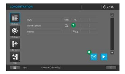
A  $(\checkmark)$  appears behind the cue "Insert sample"  $\bigcirc$ . Confirm the measurement by clicking on <OK> 8.
