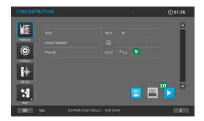
The measurement result in the units  $IU_{7.0}$  appears in the photometer display. 9. Click**START>** 10 to start the measurement procedure for the next sample.
