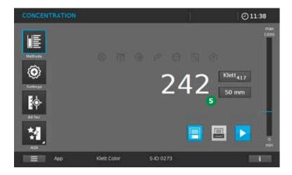
• Fill the sample solution into a 50-mm rectangular cell and insert the cell into the cell compartment.. The measurement is performed automatically and the result appears in the display 5.
