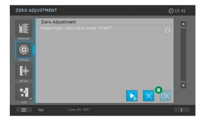
• For the zero adjustment fill a suitable rectangular cell with water for analysis.
