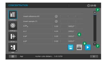
The measurement results appear in the photometer display 6.
