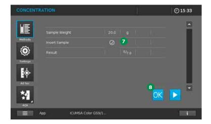
A ( $\checkmark$ ) appears behind the cue "Insert sample"  $\bigcirc$ . • Confirm the measurement by clicking on **<OK> 8**.
