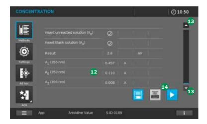
The measurement result for the Anisidine value and the absorption values  $A_1$ ,  $A_0$ ,  $A_2$  appear in the photometer display  $\Omega$ .
