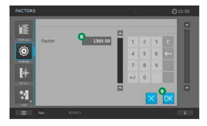
Tip on the input field "Factor" 8, enter the corrected ADMI factor, and confirm by clicking on
