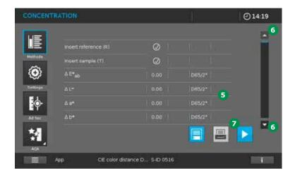
The measurement results appear in the photometer display 5.
