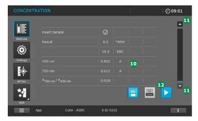
The measurement results in the units °SRM and EBC as well as the absorptions at 430 nm and 700 nm and also the quotient " $A_{700 \text{ nm}}$  /  $A_{430 \text{ nm}}$ " appear in the photometer display  $\bigcirc$ .
