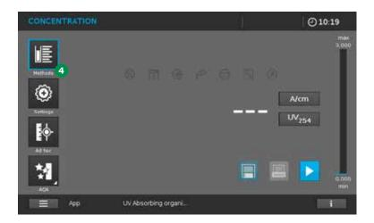
• Open the methods list (<Methods>) 4 and select Method No. 309 "UV Absorbing Organic Constituents" resp. No. 310 "UV Absorption 254".
