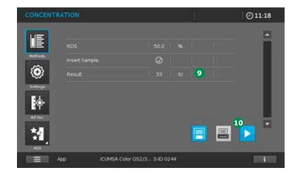
The measurement result in the units IU appears in the photometer display 9.
