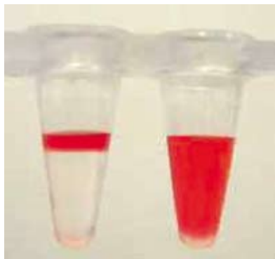
Figure 1: Experimental setup before (left) and after (right) mixing with MixMate. Left: Glycerol solutions overlayed with 1/30 volume of red colored water. Right: A completely mixed solution as indicated by the homogeneously red staining without any cords.
