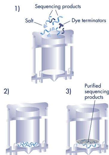
1. Add sample and injection solution to well.
