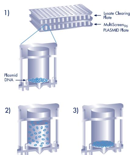
1. Using vacuum, clear lysates with the Lysate Clearing Plate. Cleared lysate is captured in the MultiScreen<sup>™</sup> PLASMID Plate.
