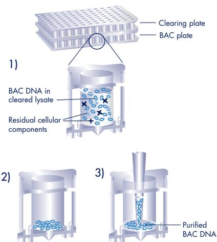
1. Assemble Clearing plate (top) and BAC plate (bottom) in manifold. Add lysate to Clearing plate and apply vacuum (6 – 8 min). Cleared lysate is collected in the BAC plate.
