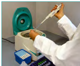
2. Cell lysis (2 mL Sample, 13.000 rpm; 37°C, 45-60 min)
