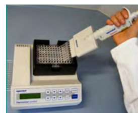
6. Washing (Removal of unbound components, 2x 1 min)
