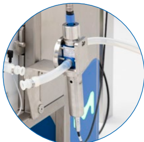
Pre-column instrumentation for conductivity and pH measurement
