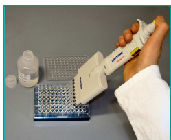
5. Enzymreaction (Coupling of an enzyme to the „Sandwich“, 20 min)
