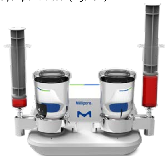
Figure 2: Decontamination accessory installed on each head of a Milliflex Oasis® pump. 50 mL of the disinfectant is kept in contact with the fluid path for 15 minutes and rinsed with 250 mL of sterile water.
