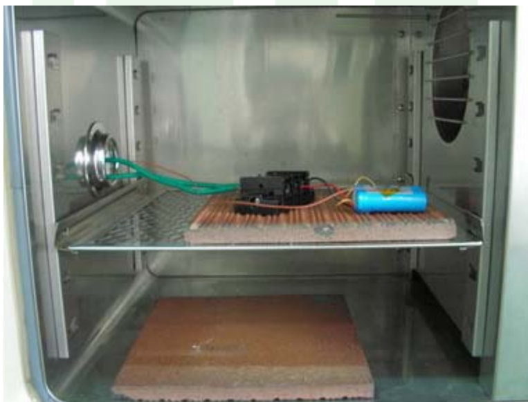
Fig.5 : External short circuit test
