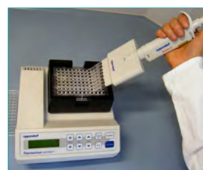
6. Washing (removal of unbound components, 2x1 min)
