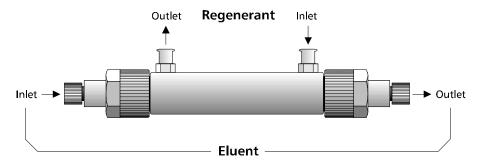
**Connecting the Regeneration flow.** The Regeneration (outer channel) flow should be connected counter-current to the Eluent (inner channel) flow (see Figure). When a SeQuant<sup>®</sup> CARS<sup>TM</sup> - Continuous Auto Regeneration System - is being installed, connect the *Regeneration Inlet* with CARS<sup>TM</sup> pump outlet and the *Regeneration Outlet* with CARS<sup>TM</sup> Cartridge inlet.
