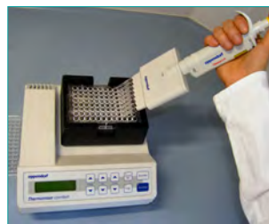
6. Washing (removal of unbound components, 2x1min)
