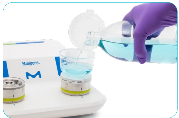
Figure 4: Filterable sample being poured into a Milliflex Oasis® filtration unit
