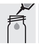
Pipette 5.0 ml of distilled water (Water for analysis EMSURE®, Cat.No. 116754, is recommended) + 5.0 ml of the sample into a 24-mm cell (do not add any reagents!), close with the screw cap, and mix. (Blank cell)
