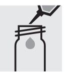
Fill approx. 10 ml of distilled water into a 24-mm cell (do not add any reagents!), close with the screw cap. (Blank cell)
