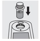
Insert the blank cell into the cell compartment. Align the mark on the cell with that on the photometer.
