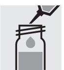
Add **5.0 ml of distilled** water (Water for analysis EMSURE®, Cat.No. 116754, is recommended) with pipette, close with the screw cap, and mix.
