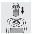
Insert the cell containing the sample into the cell compartment. Align the mark on the cell with that on the photometer. Press [Zero/Test] anew.
