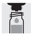
Add 3 drops of Cl<sub>2</sub>-2, close with the screw cap, and mix.
