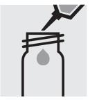
Pipette 10 ml of the sample into a 24-mm cell.
