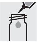
Pipette 10 ml of the sample into a 16-mm cell.
