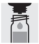
Add 2 drops of CIO<sub>2</sub>-1, close with the screw cap, and mix.
