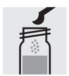
Add 1 level blue microspoon of **Cl<sub>2</sub>-1**, close with the screw cap.
