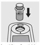
Insert the cell containing the sample into the cell compartment. Align the mark on the cell with that on the photometer. Press [Zero/Test] anew. (= T1)
