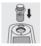
Insert the blank cell into the cell compartment. Align the mark on the cell with that on the photometer.
