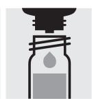
Add 3 drops of Cl<sub>2</sub>-2, close with the screw cap, and mix.
