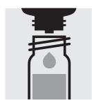
Remove the sample cell from the photometer, open, add 2 drops of Cl<sub>2</sub>-3, close with the screw cap, and mix.
