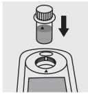
Insert anew the cell containing the sample into the cell compartment. Align the mark on the cell with that on the photometer.
