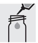
Pipette 5.0 ml of the sample into a 24-mm cell.
