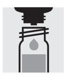
Remove the sample cell from the photometer, open, add 2 drops of Cl<sub>2</sub>-3, close with the screw cap, and mix.
