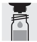
Add 2 drops of  $O_3-1$ , close with the screw cap, and mix.
