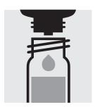
Remove the sample cell from the photometer, open, add 2 drops of Cl<sub>2</sub>-2, close with the screw cap, and mix.
