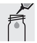
Fill approx. 10 ml of distilled water into a 24-mm cell (do not add any reagents!), close with the screw cap. (Blank cell)
