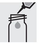
Fill approx. 10 ml of distilled water into a 16-mm cell (do not add any reagents!), close with the screw cap. (Blank cell)
