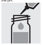
Add 10 ml of the sample with pipette, close with the screw cap, and mix.
