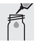
Fill approx. 10 ml of distilled water into a 16-mm cell (do not add any reagents!), close with the screw cap. (Blank cell)
