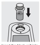
Insert the blank cell into the cell compartment.
