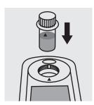
Insert the cell containing the sample into the cell compartment. Align the mark on the cell with that on the photometer. Press [Zero/Test] anew.
