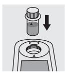
Insert anew the cell containing the sample into the cell compartment. Align the mark on the cell with that on the photometer. Press [Zero/Test] anew. (= T2)
