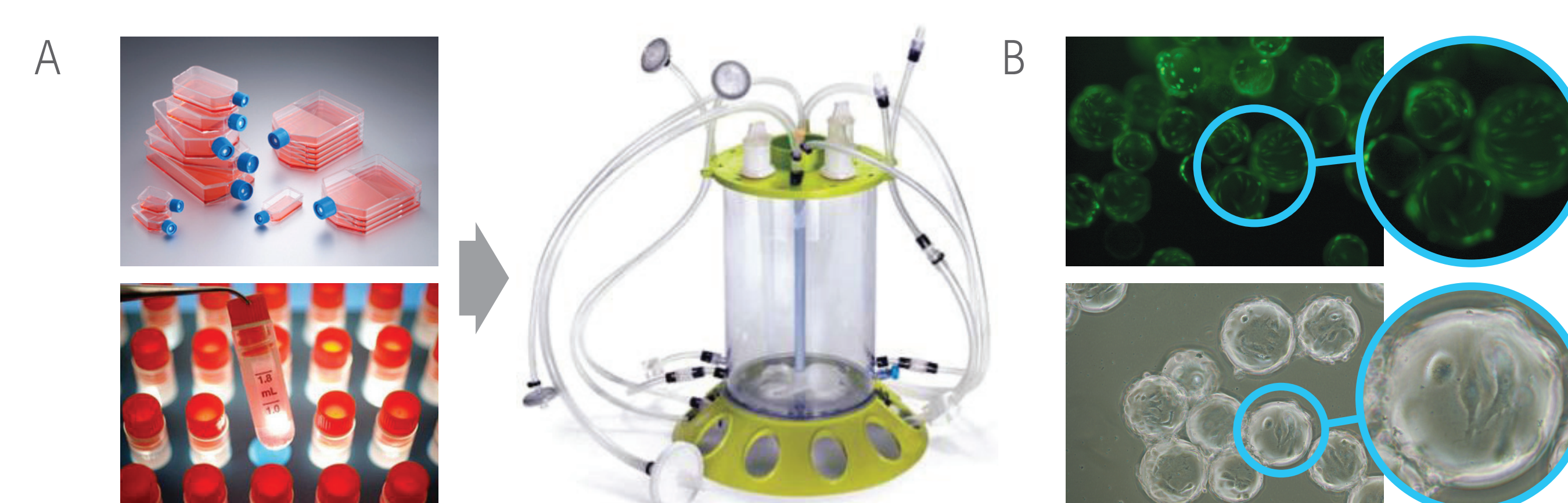
FIGURE 2. hMSCs expansion in Mobius® CellReady 3L bioreactor on microcarriers. A) hMSCs can be either expanded first on T-flasks or thawed and directly seeded into bioreactor with microcarriers; B) Morphology of hMSCs on microcarriers after expansion in the bioreactor (Upper: CellTracker Green; Lower: Bright Field).
