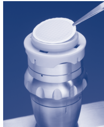
3. Incubate the membrane by lifting the membrane and transferring it onto a media plate.
